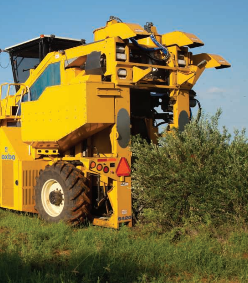
Texana Olive Ranch's olive harvester is an adapted grape harvester from Washington State. The harvester drives over the trees, and rods shake the olives free.
