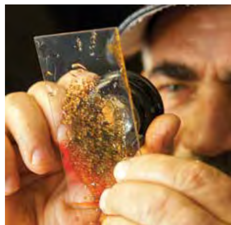
Silvio Megia checks a sample from one of LaSuCa's vacuum pans, where sugar crystals grow in the massecuite. "Working the pans is an art," Comb says.
