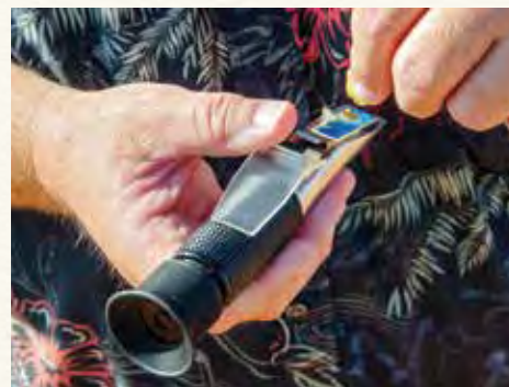
A refractor meter, which measures the brix, or percentage of sugar content, in grapes
