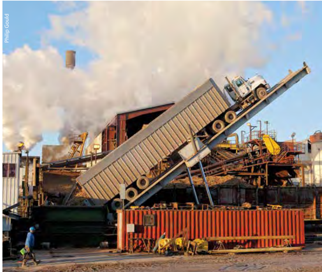
A ramp at LaSuCa tilts trucks up to 63 degrees to unload the sugarcane, which should be milled within 24 hours of harvest. The mill processes about 12,000 tons of cane a day.
